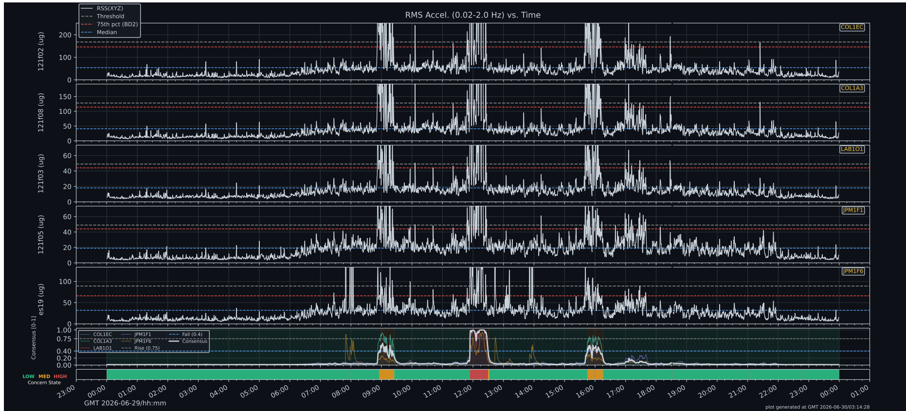
Figure 4. Daily RSS acceleration RMS below 2Hz for the same distributed SAMS sensor-head set on GMT 2026-06-29. This previous-day view provides comparison context: intermittent elevated activity is present, but it is more episodic and lacks the same sustained, coherent EVA-day interval seen on GMT 2026-06-30.
